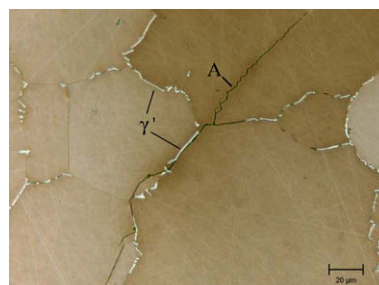
Figure 2. Top view of a crack in another nickel-aluminide coating, again after polishing away the thermally grown oxide. Specimen was cycled 40 times between 1150 and 1050 °C with 10 min at each temperature. Optical micrograph.
