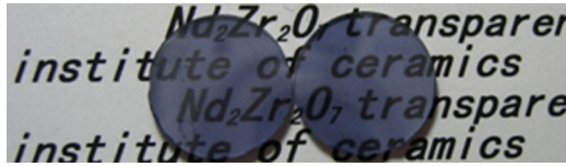
FIG. 2. (Color online) Transparent \text{Nd}_2\text{Zr}_2\text{O}_7 pellets sintered under hydrogen atmosphere at 1800 °C for 6 h (polished, thickness=1 mm).
