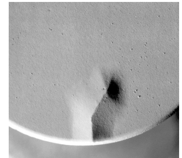
Failure typically by TBC buckling/spallation
